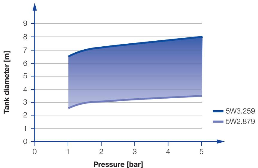
Overview of the tank diameter, depending upon the pressure of series 5W2 / 5W3
